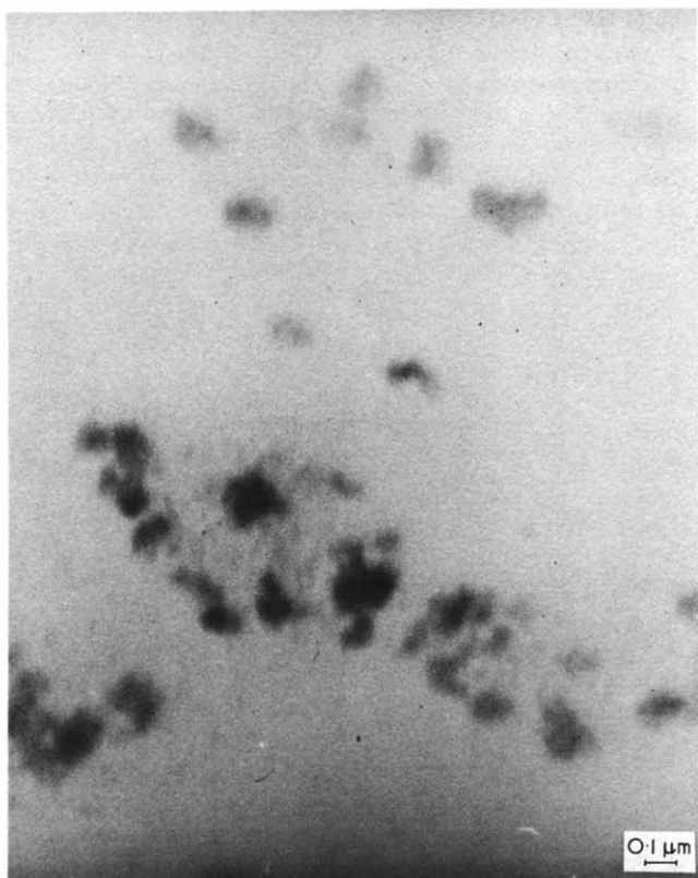
Figure 1 Tagged poly( cis -isoprene) molecules of M_v = 954\,000 in untagged poly( cis -isoprene) of the same molecular weight. Sample prepared according to Method A
